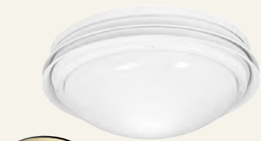
Marine II™ Low Profile Outdoor Globe 28547 New Bronze 28511 Textured Black 28438 White 28548 Weathered Bronze 26w Uses two 13w CFL bulbs (included) Rated for wet locations 10" w x 5" h
